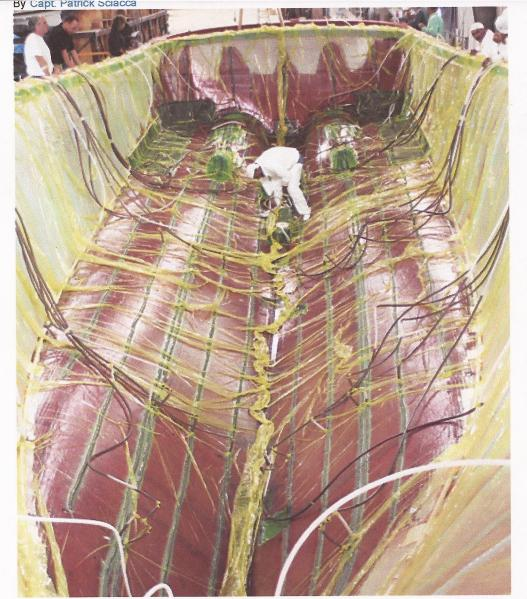
Makaira's hull is being constructed via infusion. Resin, under a vacuum, is drawn through feed lines. This process results in a lightweight, yet sturdy hull. Note the red resin being drawn up the transom.
