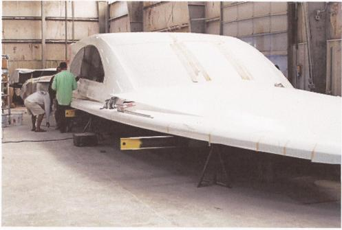
Prior to the Makaira crew's matching and securing the superstructure and the now-infused hull, the team inspects the top of the battlewagon. Interior modules are being constructed simultaneously.
