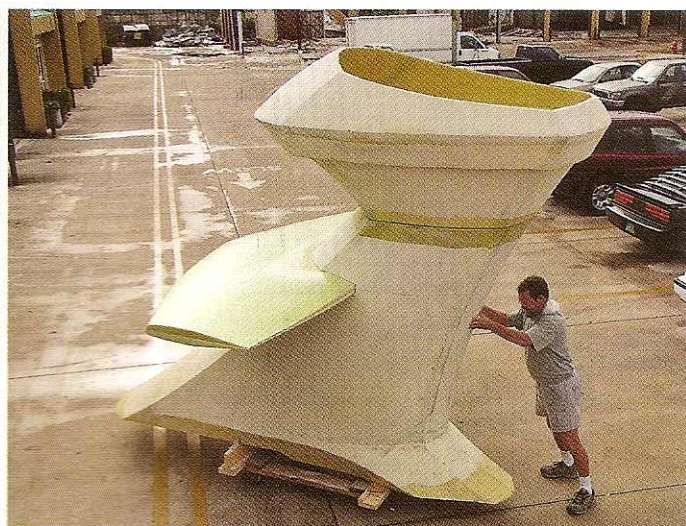
Left: Tribute Performance Boats built Double Down 's hull off a jig. Right: The composite-built tower gets dry-fit.
