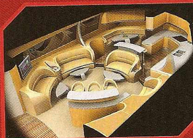
(1) Blending furniture into bulkheads maximizes interior volume.
