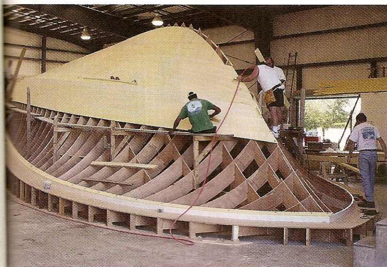
Left: Tribute Performance Boats built Double Down 's hull off a jig. Right: The composite-built tower gets dry-fit.
